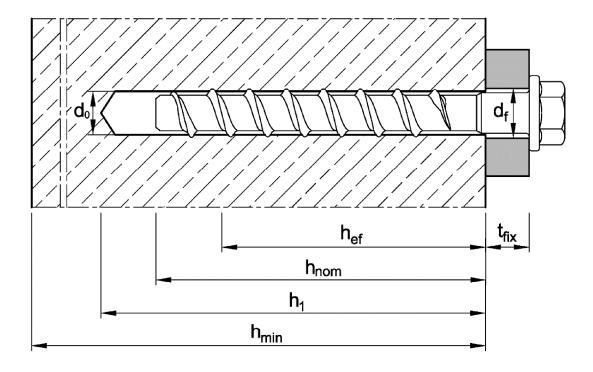
$d_0$  = nominal drill bit diameter  $h_{ef}$  = effective anchorage depth  $h_{nom}$  = nominal anchorage depth  $h_1$  = depth of the drill hole
