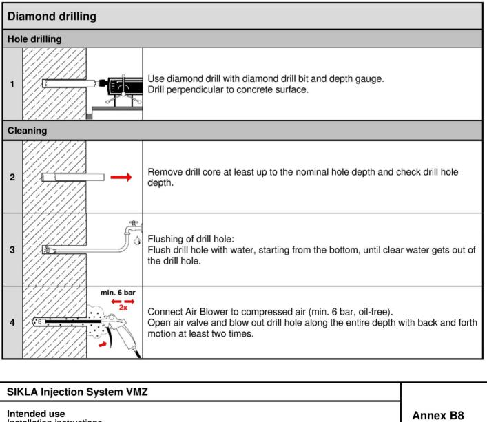
Installation instructions Hole drilling and cleaning (vacuum drill bit and diamond drill bit)
