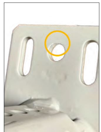
Suspension point reworked before delivery
